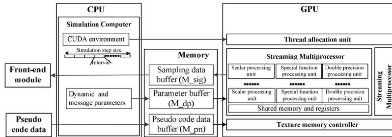
**Figure 2:** GPU accelerated signal simulation
