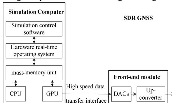
**Figure 1: SDR GNSS Simulator Architecture**
