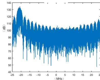
Figure 4: Spectrum of the simulated B1I signal
